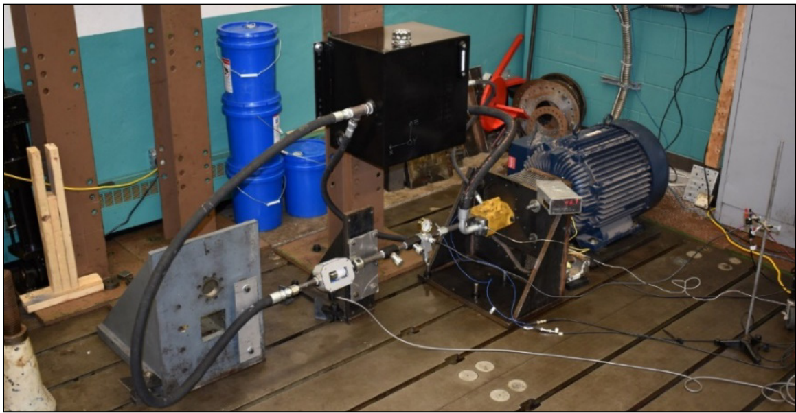
Figure 9: ISO 10767-1 Test Bench Setup
