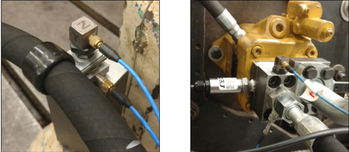
Figure 25: SBN metric data collection (Left) Pump Outlet Pressure Measurement (Right)
