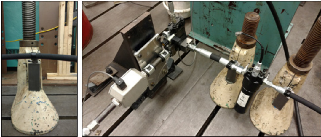
Figure 5: Hydraulic Hose Mount (Left) and End-of-Line System (Right)
